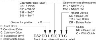
Front direct drive unit, motor on left side for 0.55kW SEW geared motor, with Free Roller and Clutch.
