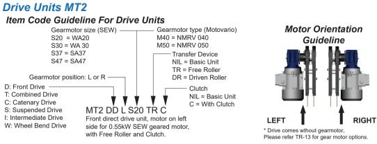
eg. Code for Basic unit; MT2 DT R M50 => Combined drive unit, motor on right side for Motovario NMRV 050 geared motor.
