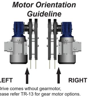
eg. Code for Basic unit; DR2 DT R M50 => Combined drive unit, motor on right side for Motovario NMRV 050 geared motor.
