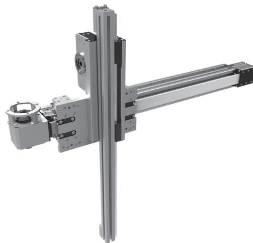
**EN** 834.HHL/835.HHL are self-aligning belt-driven linear actuators sliding on recirculating ball bearing guides. The slides are size 20. The axis have a 90x90 10 mm slot profile and a 45x45 8 mm slot profile.
