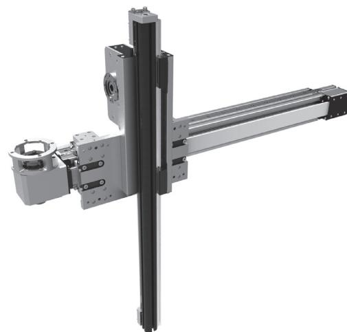
**EN** 836.HHL/837.HHL are self-aligning belt-driven linear actuators sliding on recirculating ball bearing guides. The slides are size 20. The axis have a 90x90 10 mm slot profile and a 45x45 8 mm slot profile.
