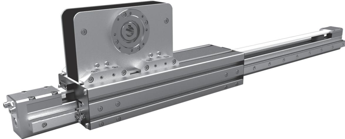
**EN** 800.045 is a belt-driven linear actuator sliding on recirculating ball bearing guides. The slides are size 20. The axis has a 45x45 8 mm slot profile.
